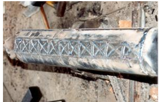
Breaker – protected by NX 100, 1 pass only
